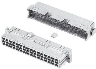
Insert the code key into one of the key ways of the female connector as shown in the drawing. Break out the corresponding area of the male shroud. Connectors coded this way can only be applied in a minimum rack spacing of 20.32 mm.
